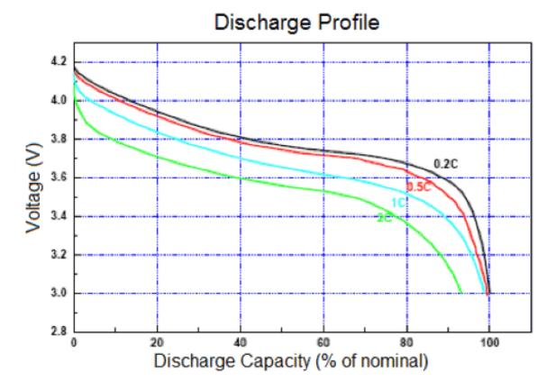
Discharge: 3.0V cutoff at room temperature.
