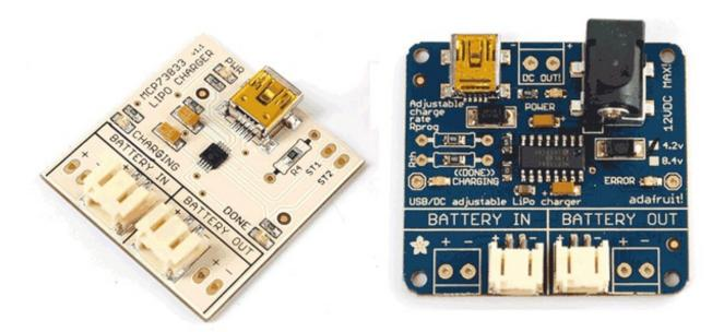
We carry two chargers in our store (at this time). A USB charger and a USB/DC charger. The USB charger is meant for charging single cells from a USB port that can provide 500mA or so. The USB/DC charger is meant for charging batteries from a USB port **or** a DC power supply up to 12V. The latter is more flexible, but more expensive because of the added circuitry.
