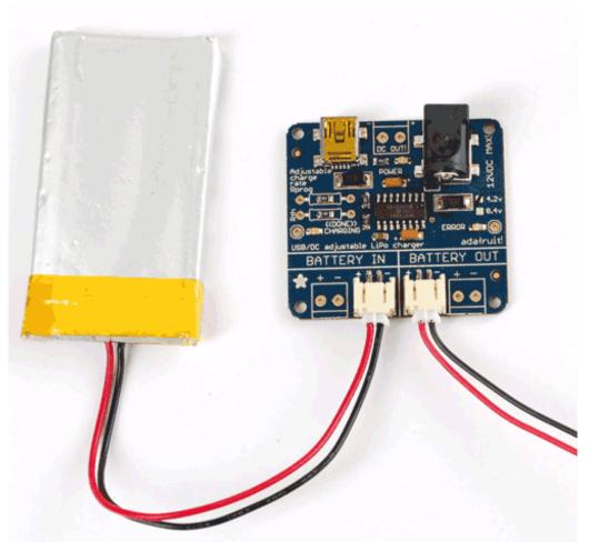
If you want to use the battery while also having it connected to the charger (less plugging and unplugging that way) you can simply use the **BATTERY OUT** connection on the right. The **IN** and **OUT** ports are connected together on the circuit board so it acts as a *pass-through* To charge, connect a power supply to the top of the board.
