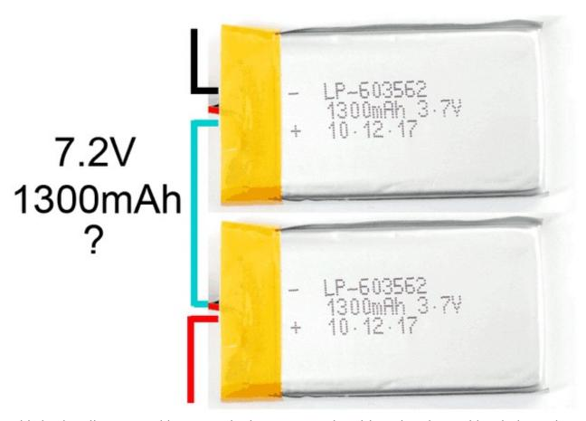
This is also discouraged because the battery wont be able to be charged in a balanced manner. You should purchase a lithium ion pack that is preassembled.
