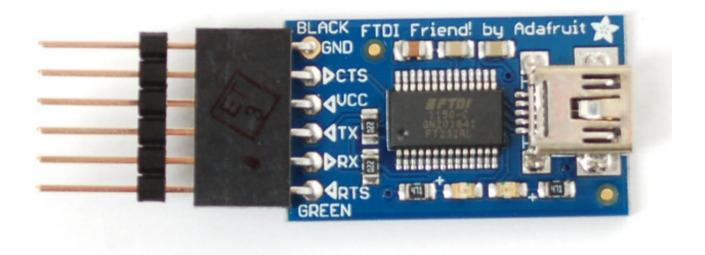
Long gone are the days of parallel ports and serial ports. Now the USB port reigns supreme! But USB is hard, and you just want to transfer your every-day serial data from a microcontroller to computer. What now? Enter the FTDI Friend!
