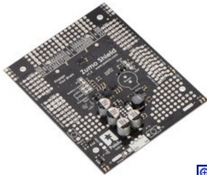
Zumo Shield for Arduino, v1.2, as it ships (assembled with surface-mount components only).
